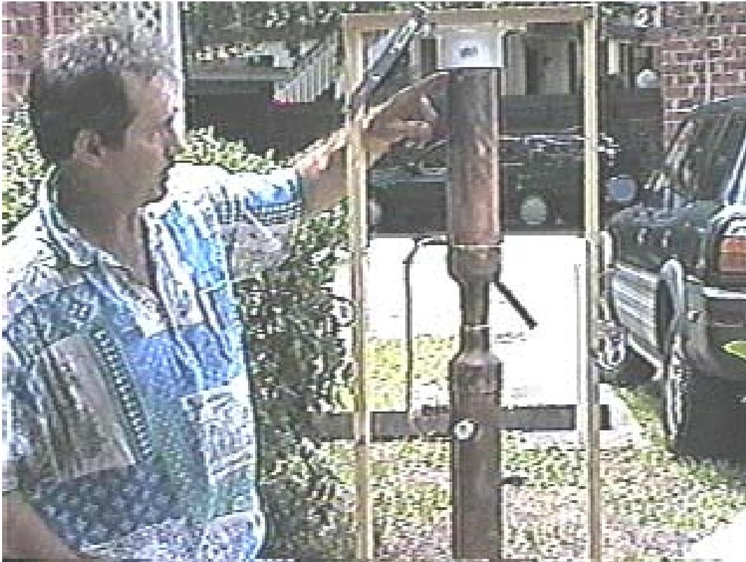
Here, I used a PVC toilet floor flange to secure the top and bottom ends of the still to the frame. The white thing in front, middle, is a white plastic plug I installed temporarily to close the hole where the temperature gauge will be installed (and keep the marbles inside).
