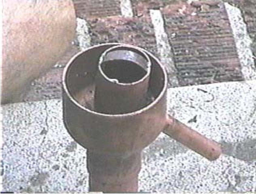
On the top of this smaller 1-1/2 inch pipe which you see in this photo is where you will attach a couple curved strips of copper to keep the marbles from the bottom section from rolling into the top section if you lay the still down into a horizontal position for carrying it. The smaller 1/2 inch pipe on the lower right of this photo is the high-proof fuel outlet.
