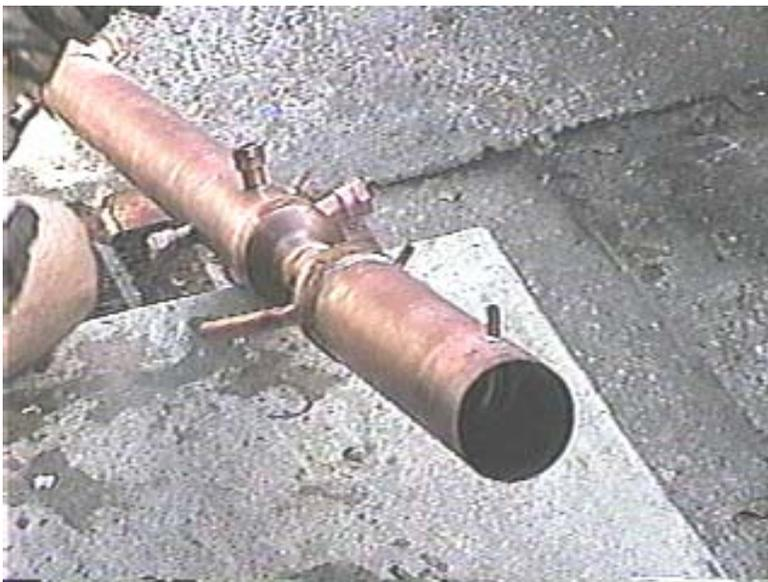
Top of condenser section with coil inserted.
