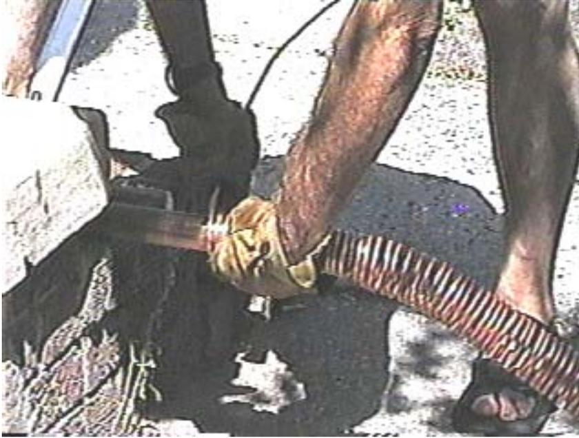
Here in the above photo, I am standing on the 1-1/2" pipe I am using as a rolling jig, and have it pinched up against the back step of my house, to hold it securely. With my left hand (the hand in front, wearing a leather glove), I am twisting the coil away from me, while the right hand guides the straightened-out copper tubing onto the newly-formed coil.
