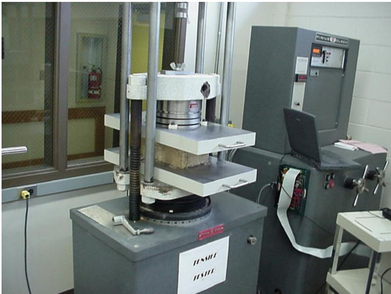
**Figure 5** Compression Test Set Up
