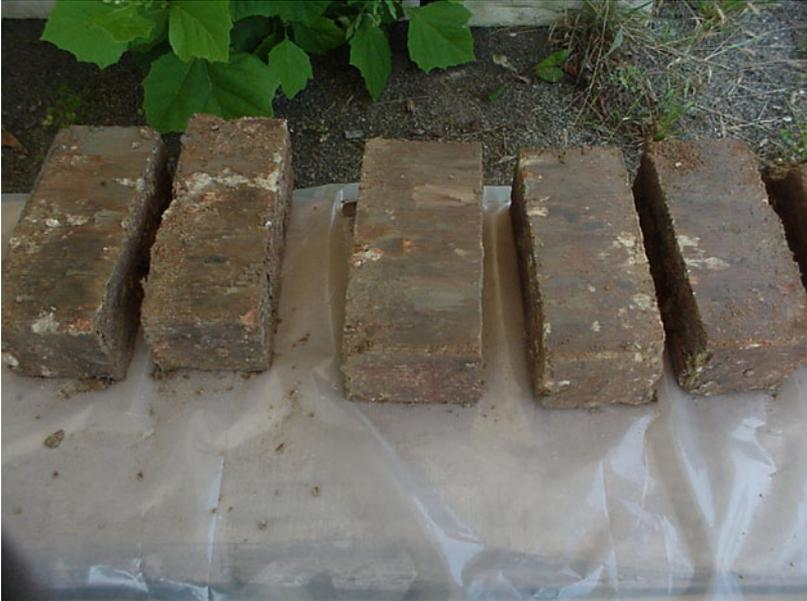
**Figure 4** Some Compressed Earth Blocks
