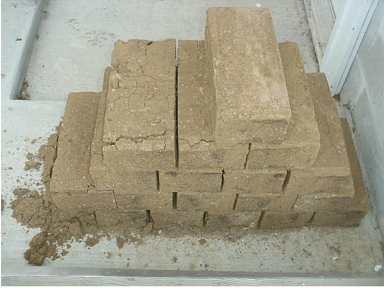
**Figure 6** Crushing of Bottom Blocks After Exposure to Snow and Rain (after 3 months)
