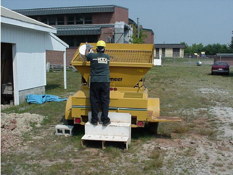
**Figure 2** Loading Hopper of the Press with Soil
