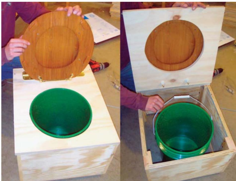
Keep the metal receptacle handle (the bail) on back side of the toilet as shown above right. The receptacle should protrude above the hinged plywood top  $\frac{1}{4}$ " to  $\frac{1}{2}$ " as shown above left. Adjust feet accordingly.
