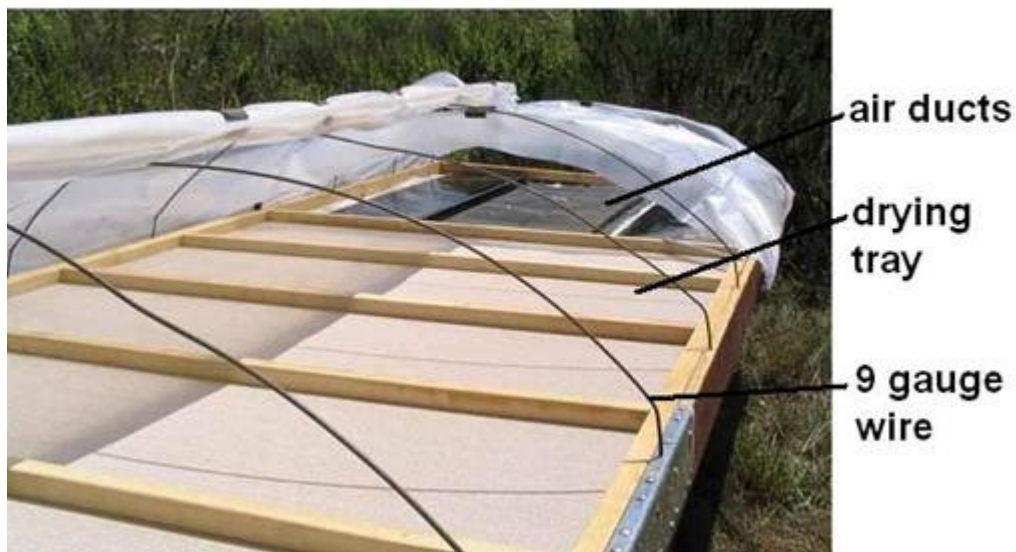
Figure 6. Air ducts convey heat under drying trays.
