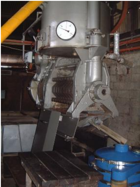
Figure 6: Rosedowns Maxoil press. Photo: Tony Swetman.
