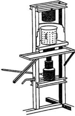
**Figure 4: Oil press with a hydraulic jack**
