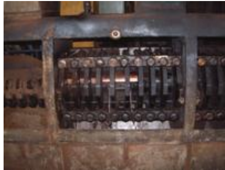
Figure 7: Typical view of cage or barrel of an expeller. Photo: Tony Swetman.
